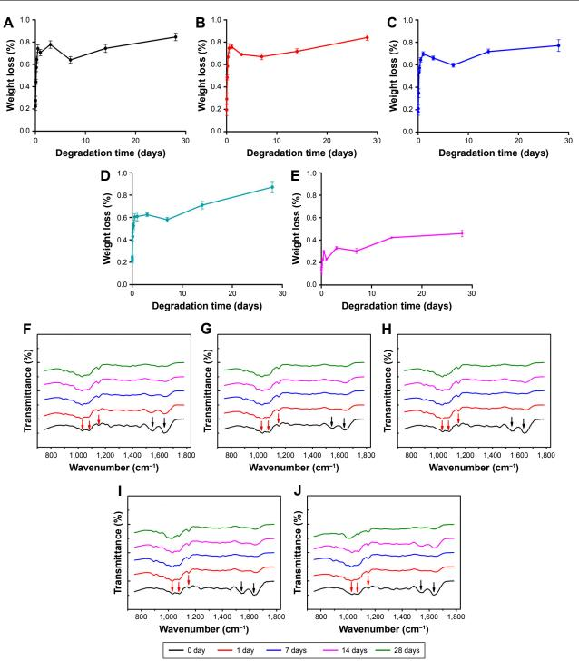
Figure 6 (A–E) Degradation rate of CS/G and Ag-containing nanocomposite coatings in PBS under sterile condition (n=4) and (F–J) ATR-FTIR spectra of CS/G and Agcontaining nanocomposite coatings after degradation in PBS at specific times: 0, 1, 7, 14, and 28 days (red arrows: peaks corresponding to chitosan; black arrows: peaks corresponding to gelatin): (A and F) Ag-0, (B and G) Ag-1, (C and H) Ag-III, and (E and J) Ag-IV.
