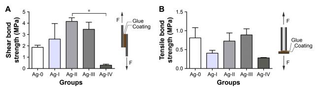
Figure 5 Bar graph of the (A) shear and (B) tensile bond strength of CS/G and Ag-containing nanocomposite coatings on titanium surface (n=3; \*P<0.05). Abbreviations: CS/G, chitosan/gelatin; F, force.
