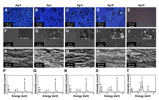
Figure 2 (A–E) The fluorescence images, (F–J) SEM images of surface with low and high magnification, (K–O) SEM images of cross-section, and (P–T) EDS spectra of CS/G and Ag-containing nanocomposite coatings (square: C, circle: O, triangle: Au, inverted triangle: CI, star: Ag, diamond: Ti). Abbreviations: SEM, scanning electron microscopy; EDS, energy-dispersive X-ray spectrometry; CS/G, chitosan/gelatin.
