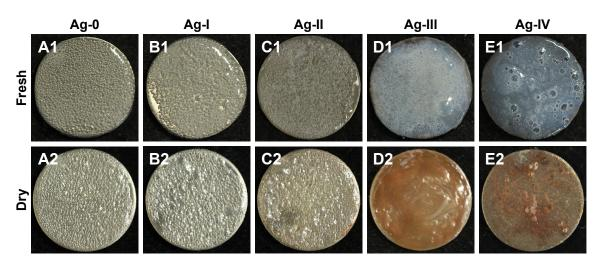
Figure I The optical photographs of fresh (AI–EI) and dry (A2–E2) CS/G and Ag-containing nanocomposite coatings. Abbreviation: CS/G, chitosan/gelatin.
