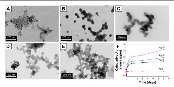
Figure 4 TEM images of the released nanoparticles and calculative release profiles of Ag ions from CS/G and Ag-containing nanocomposite coatings in PBS: (A) Ag-0, (B) Ag-1, (C) Ag-11, (D) Ag-111, (E) Ag-IV, and (F) release profile. Abbreviations: TEM, transmission electron microscopy; CS/G, chitosan/gelatin; PBS, phosphate-buffered saline.
