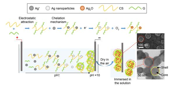
Scheme I Fabrication process of Ag-containing nanocomposite coating via EPD. Ag-containing nanoparticles were formed as shown in the SEM result. TEM results revealed a core-shell-like structure of the released nanoparticles.
