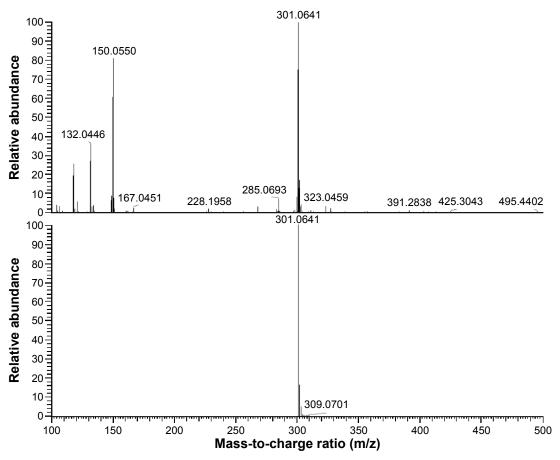
**Figure S3** Matrix-assisted ionization-high-resolution mass spectrum for RBC-2008. **Note:** Predicted spectrum for  $C_{15}H_{12}N_2O_3S+H$  is shown at the bottom.
