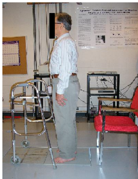
Figure 1 Participant in two-limb standing position on the force plate for balance testing.
