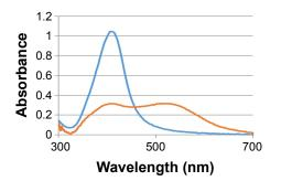
Figure S5 AgNPs suspended in bacteria nutrient broth (orange line) and in sodium citrate 1 mM solution (blue line). In the first case, as broader peak shows, nanoparticles aggregation occurs.
