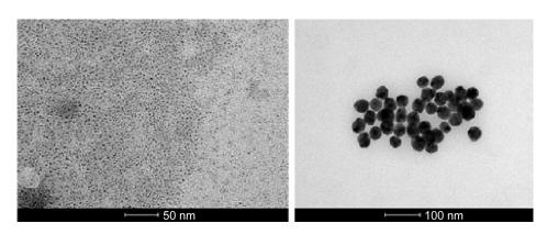
Figure S6 TEM images of CSNPs, scale bar: 50 nm (left) and SNPs scale bar: 100 nm (right). Abbreviations: CSNPs, colloidal silver nanoparticles; SNPs, silver nanoparticles; TEM, transmission electron microscopy.
