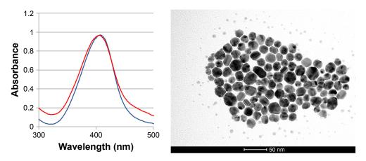
Figure S4 AgNPs stability evaluated by UV-vis spectroscopy in citrate 1 mM before (red line) and after (blue line) the lyophilization (left). TEM image of lyophilized AgNPs (right).
