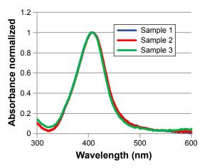
Figure S1 Plasmon band position of three samples of AgNPs by UV-vis absorption spectroscopy. Abbreviations: AgNPs, silver nanoparticles; UV-vis, ultraviolet-visible.
