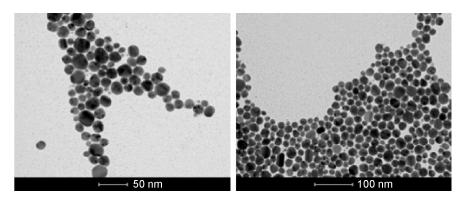
Figure S2 TEM images of AgNPs suspended in water, scale bar: 50 nm (left) and 100 nm (right). Abbreviations: AgNPs, silver nanoparticles; TEM, transmission electron microscopy.
