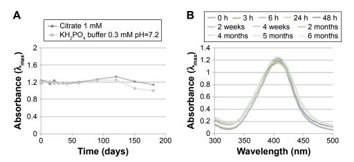
**Figure S3** Long-term stability of AgNPs in citrate buffer 1 mM and phosphate buffer 0.3 mM (pH 7.2) (**A**) expressed as absorbance at  $\lambda_{max}$  variations as function of time; plasmon band position of AgNPs by UV-vis absorption spectroscopy (**B**). **Abbreviations:** AgNPs, silver nanoparticles; UV-vis, ultraviolet-visible.
