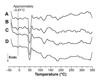
Figure 5 DSC scans of the F11 NLC and copper(II) complex-loaded NLCs, (A) F11, (B) F11.1, (C) F11.2, and (D) F11.3.
