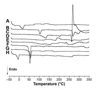
Figure 4 DSC scans of free copper(II) complexes I, 2, and 3 and the components used in preparation of NLCs: (A) polyoxyl-40 hydrogenated castor oil (PEG-40); (B) cetyltrimethylammonium bromide (CTAB); (C) [CuCl<sub>2</sub>(INH)<sub>2</sub>]·H<sub>2</sub>O (1); (D) [Cu(NCS)<sub>2</sub>(INH)<sub>2</sub>]·5H<sub>2</sub>O (2); (E) [Cu(NCO)<sub>2</sub>(INH)<sub>2</sub>]·4H<sub>2</sub>O (3); (F) poloxamer 407 (P-407); (G) polyoxyethylene 40 stearate (E-40); (H) caprylic/capric triglyceride (CCTG).
