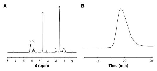
Figure I Characterization of copolymer CA-PLGA-TPGS: (A) typical <sup>1</sup>H NMR spectra and (B) gel permeation chromatographic analysis. Abbreviations: CA, cholic acid; PLGA, poly(lactide-co-glycolide); TPGS, D- $\alpha$ -tocopheryl polyethylene glycol 1000 succinate; <sup>1</sup>H NMR, <sup>1</sup>H nuclear magnetic resonance.
