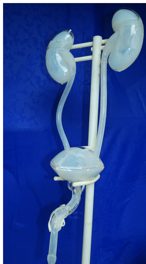
Figure 2 The male urinary-system-simulating physical model.
