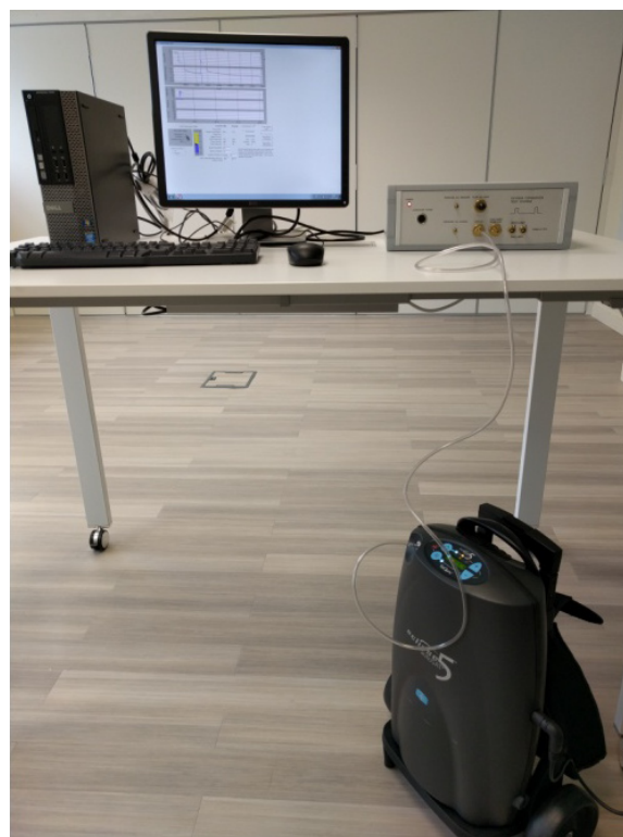
Figure 1 Eclipse 5 portable oxygen concentrator connected to the test system.
