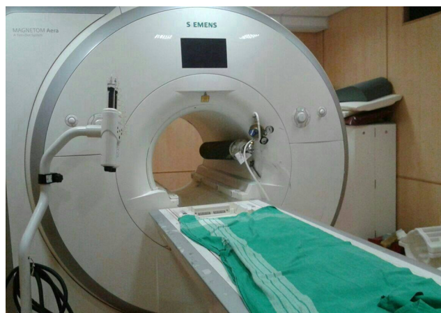
Figure 6 3 T MRI systems – oxygen tank was pulled into the magnet.
