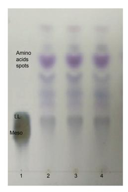
Figure 2 TLC analysis of whole-cell hydrolysate of SUK 25.
