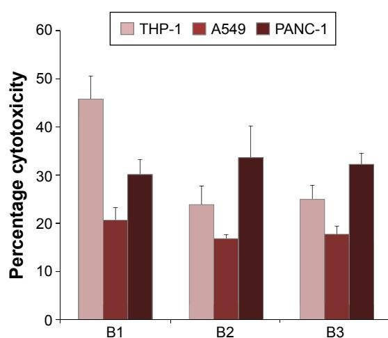
**Figure 3** Percentage cytotoxicity of gold–silver bimetallic nanoparticles at 30 μg/mL against human cell lines.
