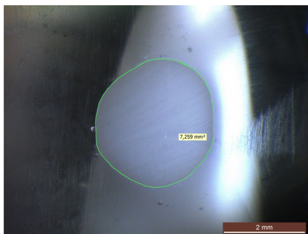
Figure 7 Measurement of a cut state-of-the-art Y-TZP FDP core under light microscope.
