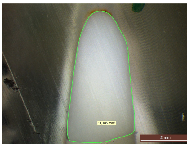
Figure 6 Measurement of a cut split-file Y-TZP FDP core under light microscope. Notes: The figure shows the cross-section area of the connector between the central incisor and pontic.
