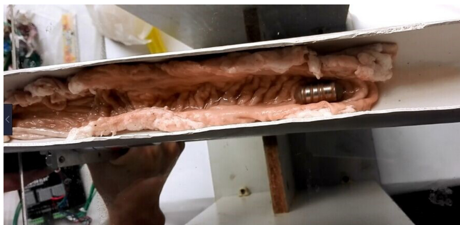
Figure 7 Measurement setup of translational motion time.
