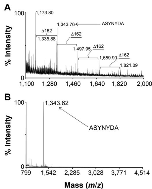
**Figure 3** Characterization of NPs-DCM-ASYNYDA nanoparticles by MALDI-TOF/TOF analysis.
