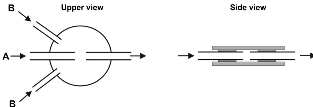
**Figure 2** Schematic drawing of microfluidic precipitation device.
