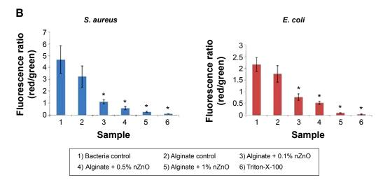
Figure 7 Evaluation of antibacterial activity of alginate hydrogel/nZnO composite bandages.
