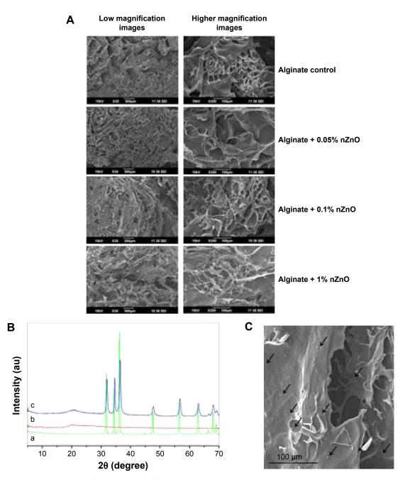
$\label{eq:Figure 2} Figure \ 2 \ Physico-chemical \ charecterisation \ of \ alginate \ hydrogel/nZnO \ composite \ bandages.$
