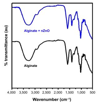
Figure 3 FTIR image of alginate control and alginate + nZnO bandages. Abbreviations: FTIR, Fourier transform infrared spectroscopy; nZnO, zinc oxide nanoparticles; au, arbitrary units.
