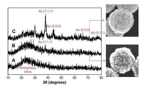
Figure 3 X-ray diffraction analysis of SGNS: (A) Au-deposited silica, (B) SGNS prepared with 0.38 mM of Au salts, (C) SGNS prepared with 1.52 mM of Au salts. The upper and lower inserts are the magnified SEM images of f-SGNS and p-SGNS, respectively.
