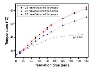
Figure S2 Temperature increment of SGNS solution with the increase of exposure times of NIR light (820 nm, 30 W/cm<sup>2</sup>). As-prepared samples (silica core =120 nm) exhibited the different thickness of the gold layer. In reference, the temperature increment by p-SGNS was provided for the comparison. Abbreviations: SGNS, silica–gold nanoshell; p-SGNS, partially covered-silica–gold nanoshell; NIR, near infra-red.
