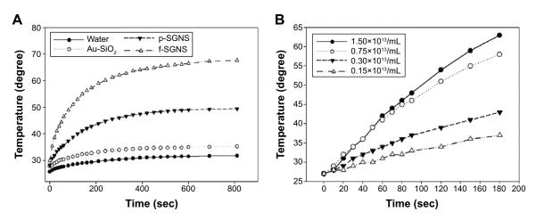
Figure 5 Temperature change of SGNS solution with increasing exposure times of NIR irradiation: (**A**) as-prepared samples with different surface coverage of Au clusters, including pure water, (**B**) different dilution ratio (×1, ×2, ×5, ×10) of original SGNS solution (1.5×10<sup>13</sup>/mL). **Abbreviations:** SGNS, silica–gold nanoshell; p-SGNS, partially covered-silica–gold nanoshell; f-SGNS, fully covered-silica–gold nanoshell; sec, seconds; NIR, near infra-red.
