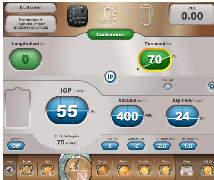
Figure 1 The machine panel display of the Quadrant Removal Setting (Quadrant Removal Step Button enlarged) in the procedure step toolbar shows a –2 vacuum rise with linear control (angled line) of torsional amplitude.
