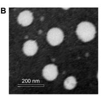
Figure 5 Characterization of CM-Ns. Notes: (A) Particle size and size distribution and (B) a TEM image. Abbreviations: CM, curcumin; CM-Ns, CM-nanoemulsions; TEM, transmission electron microscope.
