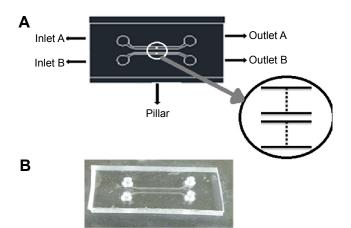
**Figure 2** Photographs of (**A**) photomask for photoresist process for SU-8 molding, inset photo shows the amplified image of pillars in the channel, and (**B**) fabricated PDMS microfluidic chip on glass slide by using  $O_2$  plasma. **Abbreviation:** PDMS, polydimethylsiloxane.
