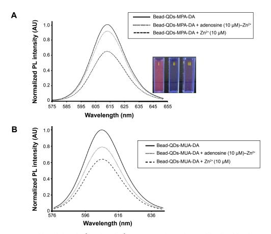
Figure 5 Normalized PL spectra of QDs-DA, QDs-DA-Zn<sup>2+</sup>, and QDs-DA-Zn<sup>2+</sup>-adenosine with surface modification by (**A**) MPA and (**B**) MUA. Inset photograph depicts the (i) QDs-DA, (ii) QDs-DA-Zn<sup>2+</sup>, and (iii) QDs-DA-Zn<sup>2+</sup> with adenosine system. **Abbreviations:** PL, photoluminescence; QDs, quantum dots; DA, dopamine; MPA, mercaptopropionic acid; MUA, mercaptoundecanoic acid; AU, atomic units.
