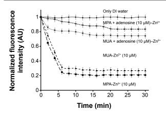
Figure 7 Fluorescence intensity variations of QDs as a function of time after injection of 10  $\mu mol \ L^{-1} \ Zn^{2*}$  solution.
