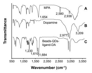
**Figure 3** FTIR spectra of **(A)** MPA, **(B)** L-DA, and **(C)** beads-QDs-DA. **Abbreviations:** FTIR, fourier-transform infrared; MPA, mercaptopropionic acid; DA, dopamine; QDs, quantum dots.
