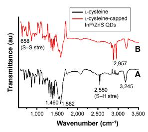
Figure 2 The FTIR spectra of (A) free L-cysteine and (B) L-cysteine-capped InP/ ZnS QDs.
