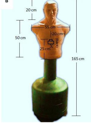
Figure 1 The position of the light (A) and accelerometer (B) in the dummy. Abbreviation: X, accelerometer.
