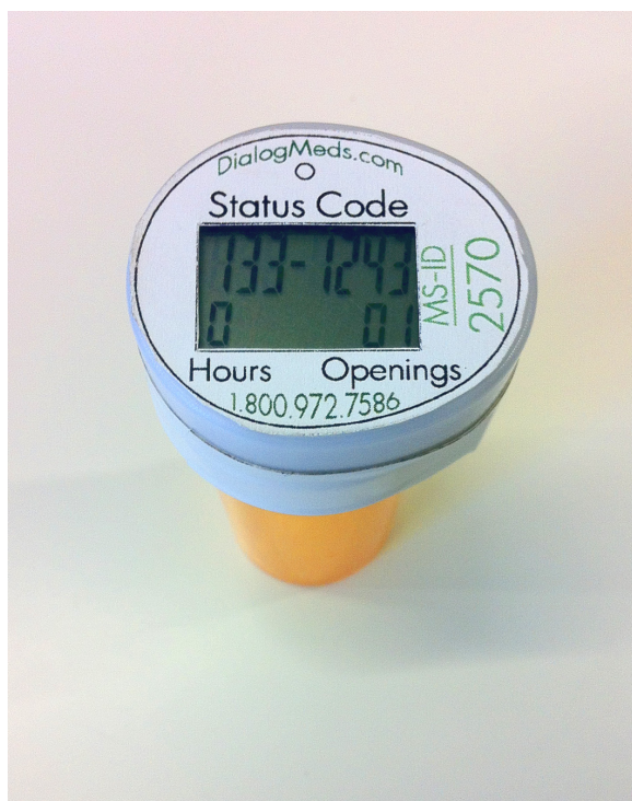
Figure 1 Illustration of an automated pill cap to monitor pill adherence in patients with bipolar disorder (BD).
