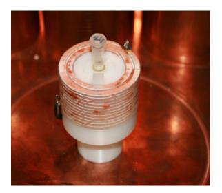
Figure 4 Transmit and receive setup of a magnetic particle spectrometer.
