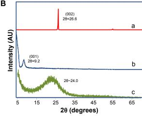
Figure 3 Characterizations of RGO by FTIR and XRD.
