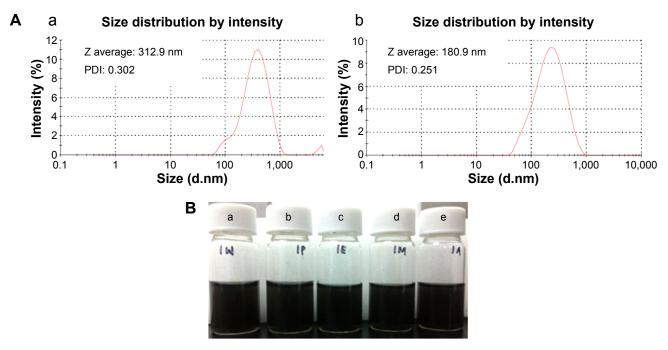
Figure 7 DLS characterization and photograph of RGO dispersion in different solvents.
