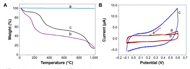
Figure 8 Thermal and electrochemical analysis of RGO using TGA and cyclic voltammetry.
