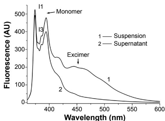
**Figure 5** Fluorescence spectra for the suspension and supernatant. Coexistence of a monomer peak and an excimer peak indicates that pyrene exists in suspension in the two states. The absence of an excimer peak in the supernatant indicates the absence of pyrene nanoparticles.
