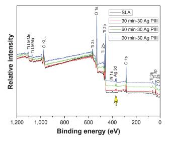
Figure 2 The typical XPS spectra of four different groups. Notes: The yellow arrow indicates the Ag 3d doublet two peaks.
