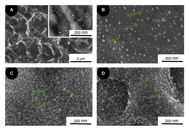
Figure I SEM photographs of (A) the untreated SLA surface and higher magnification image inserted, (B) 30 min-30 Ag PIII, (C) 60 min-30 Ag PIII, (D) 90 min-30 Ag PIII. Notes: (A) Particles around 15 nm scattered in particles around 5 nm; (B) particles with sizes around 10-25 nm; (C) particles fused together. The peak of the particle size is greater than 40 nm.
