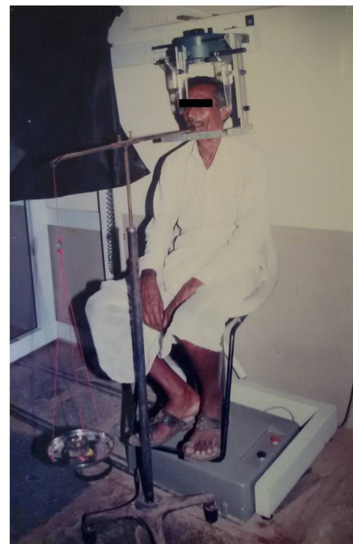
Figure 8 Force applied on denture base using T-device.
