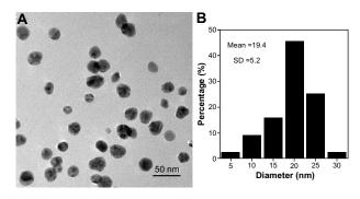
Figure I Morphology and size of the silver nanoparticles. (A) Transmission electron microscopic image of silver nanoparticles dispersed on a transmission electron microscopy copper grid. (B) A histogram showing size distribution of the silver nanoparticles.
