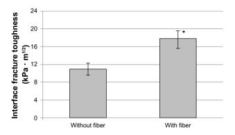
Figure 7 Fracture toughness of the titanium–poly(methyl methacrylate) interface as a function of fiber application. Data presented as means  $\pm$  standard error of mean; n=9. Note: \*p<0.001 (compared to without fiber).
