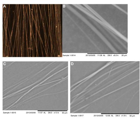
Figure 4 (A) Stereomicroscope image of unidirectional fibers at 8× magnification, (B–D) scanning electron microscopy images of three samples.
