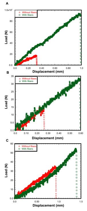
Figure 5 Load versus displacement graphs of titanium–poly(methyl methacrylate) samples under (A) tension, (B) mixed, and (C) shear load.
