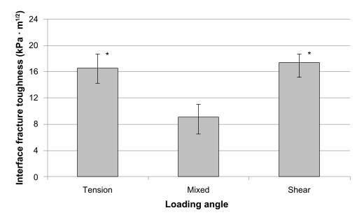
Figure 6 Fracture toughness of the titanium-poly(methyl methacrylate) interface as a function of loading angle. Data presented as means ± standard error of mean; n=6. Note: \**P*<0.01 (compared to mixed).
