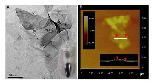
Figure 2 (A) Transmission electron microscopic images of carboxylated graphene oxide (inset: graphene dispersion in phosphate-buffered saline) and (B) atomic force microscopic images of carboxylated graphene oxide.
