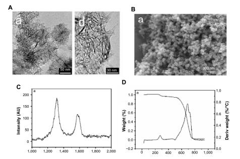
Figure SI Characterization of carbon nanohorns prepared in an atmosphere of air.
