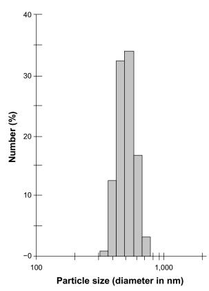
Figure S4 Single-walled carbon nanohorns particle size distribution in aqueous suspension.
