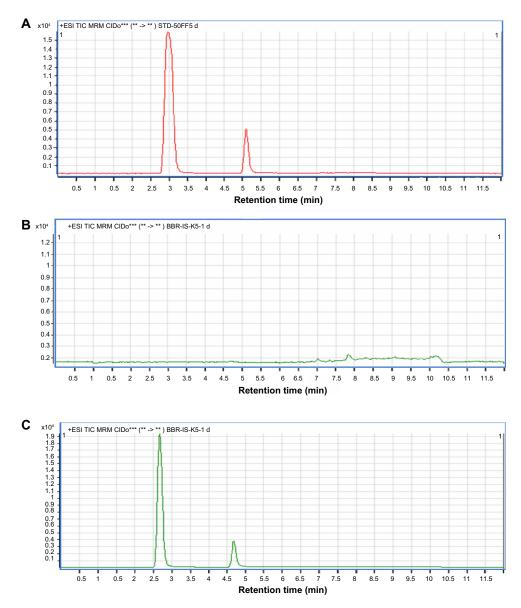
Figure 5 The selected reactions monitoring chromatograms for berberine. Notes: (A) Standard berberine and internal standard in control plasma. (B) Blank plasma. (C) Plasma sample after intragastric administration.
