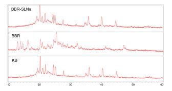
Figure 3 X-ray diffraction of berberine solid lipid nanoparticles. Abbreviations: BBR, berberine; BBR-SLNs, berberine solid lipid nanoparticles; KB, blank nanoparticles without drug prepared with the same preparations of berberine solid lipid nanoparticles.
