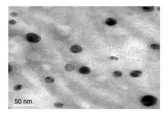
Figure 2 Microphotograph of berberine solid lipid nanoparticles.
