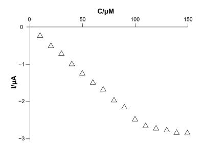
Figure 7 Calibration curve for the reduction current and concentration of epinephrine in phosphate-buffered saline (pH 7.0). Applied potential -0.07 V.
