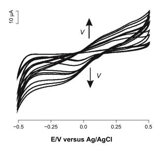
Figure 4 Cyclic voltammograms of biosensor immersed in  $10^{-5}$  M solution of epinephrine (supporting electrolyte phosphate-buffered saline, pH 7.0) registered at different scan rates, from 0.05 to 1.00 V per second.
