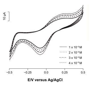
Figure 5 Cyclic voltammograms of biosensor immersed in epinephrine solutions of different concentrations ( $1 \times 10^{-5}$  M,  $2 \times 10^{-5}$  M,  $3 \times 10^{-5}$  M, and  $4 \times 10^{-5}$  M).
