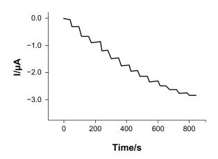
Figure 6 Amperometric response of tyrosinase-based biosensor to epinephrine in 0.1 M phosphate-buffered saline solution (pH 7.0) under constant stirring, with levels increasing in 20  $\mu$ M increments. Applied potential –0.07 V.
