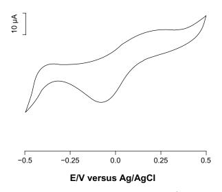
Figure I Cyclic voltammogram of biosensor immersed in  $10^{-5}$  M solution of epinephrine (supporting electrolyte phosphate-buffered saline, pH 7.0). Scan rate 50 mV per second.
