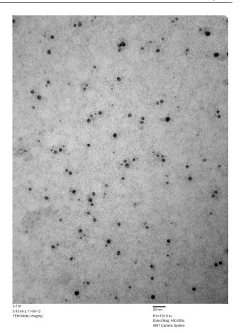
Figure I TEM analysis of silver nanoparticles.
