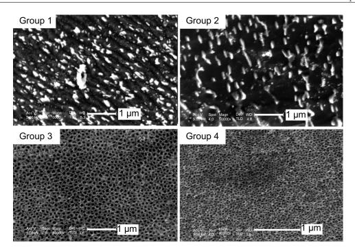
**Figure 1** SEM images of the surface morphologies of the four groups: mechanically polished titanium sheet (group 1), acid-etched titanium sheet (group 2), TiO<sub>2</sub> nanotube arrays anodized at 20 V (group 3), and TiO<sub>2</sub> nanotube arrays anodized at 10 V (group 4). **Abbreviations:** SEM, scanning electron microscopy; TiO<sub>3</sub>, titanium oxide.
