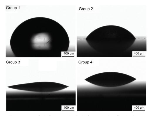
**Figure 4** Schematic of the water contact angle for the four groups: mechanically polished titanium sheet (group 1), acid-etched titanium sheet (group 2),  $TiO_2$  nanotube arrays anodized at 20 V (group 3), and  $TiO_2$  nanotube arrays anodized at 10 V (group 4). **Abbreviation:**  $TiO_2$ , titanium oxide.
