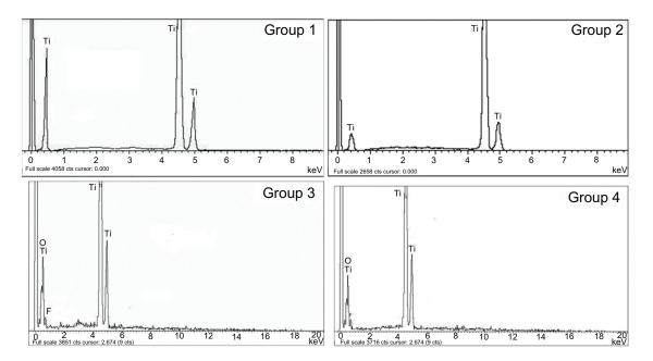
**Figure 2** EDX spectra of the four groups, including the mechanically polished titanium sheet (group 1), acid-etched titanium sheet (group 2), TiO<sub>2</sub> nanotube arrays anodized at 20 V (group 3), and TiO<sub>2</sub> nanotube arrays anodized at 10 V (group 4). **Abbreviations:** EDX, energy dispersive X-ray; TiO<sub>3</sub>, titanium oxide.
