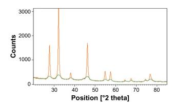
Figure 9 X-ray diffraction spectrum of green-synthesized silver nanoparticles.
