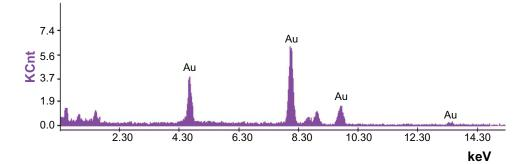
Figure 7 Energy dispersive X-ray spectrum of gold nanoparticles. Abbreviation: Au, gold.
