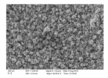
**Figure 4** Scanning electron microscopy image of green silver nanoparticles synthesized by reduction of aqueous AgNO<sub>3</sub> ions using *Chrysopogon zizanioides* extract. **Abbreviations:** EHT, extra high tension; Mag, magnification; WD, working distance.
