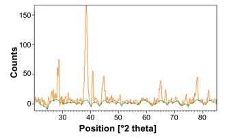
Figure 10 X-ray diffraction spectrum of green-synthesized gold nanoparticles.
