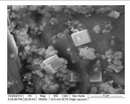
Figure 5 Scanning electron microscopy image of green gold nanoparticles synthesized by reducing aqueous  $AuCl_4^-$  ions using *Chrysopogon zizanioides* extract. Abbreviations: Mag, magnification; WD, working distance; ETD, Everhart-Thornley detector; Vac, vacuum; HV, high voltage; Det, detector.
