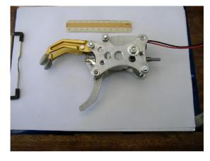
Figure I Mechanical structure of the prosthetic hand. Note: A 10 cm ruler is shown as a reference.
