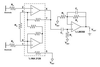
Figure 2 Front end of the electromyograph.
