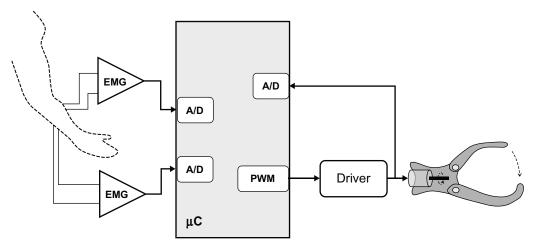
Figure 3 Block diagram of the control circuit of the prosthesis. Abbreviations: A/D, analog to digital converter; EMG, electromyograph; PWM, pulse-width modulated.
