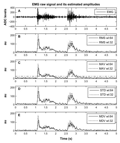
Figure 4 Example of raw electromyograph (EMG) (A) along with the real-time measurement of muscle activity as provided by the root mean square (RMS) (B), mean absolute value (MAV) (C), standard deviation (STD) (D), and mean absolute differential value (MDV) (E) operators.
