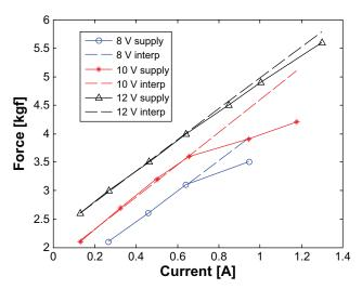
Figure 6 Measured grasp force versus absorbed current at different supply voltages. Abbreviation: interp, interpolation.
