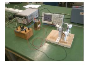
$\textbf{Figure 5} \ \ \text{Measurement setup for prosthesis characterization}.$
