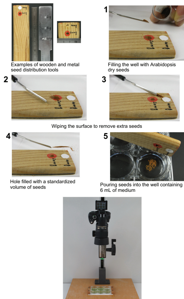
Figure S1 Method for distributing equal amounts of Arabidopsis seeds into a multiwell plate and image acquisition setup.
