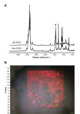
Figure II (A) Raman spectra obtained via confocal microscopy of raw dipalmitoylphosphatidylcholine (DPPC) and formulated spray-dried (SD) DPPC at 100% pump rate. The colored arrowhead shows the mapped bands. (B) Raman spectroscopic mapping showing the area of the Raman bands between 1400 and 1520 cm<sup>-1</sup> (brighter-red colors indicate greater area) superimposed on a bright-field optical image of the surface of a particle of formulated SD DPPC (100% pump rate).
