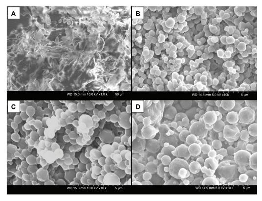
Figure 2 (A–D) Scanning electron micrographs of raw dipalmitoylphosphatidylcholine (DPPC) and spray-dried 100 DPPC particles at three pump rates. (A) Raw DPPC, magnification 1000x; (B) DPPC particles at 10% (low P) pump rate, magnification 10,000x; (C) DPPC particles at 50% (medium P) pump rate, magnification 10,000x; (D) DPPC particles at 100% (high P) pump rate, magnification 10,000x.
