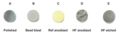
**Figure 1** Change in surface appearance from the different treatment methods. **Abbreviations:** Ref, reference; HF, hydrofluoric acid.
