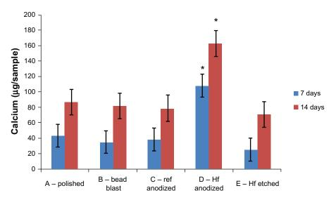
Figure 6 Calcium deposition by osteoblasts on the samples of interest to the present study. Notes: Values are mean  $\pm$  SEM, N = 3. \*P < 0.01 compared to all others at the same time period. For all samples, a significantly (P < 0.01) greater amount of calcium was found at increasing time periods.
