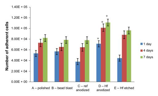
Figure 3 The number of adherent cells at all time points on the samples of interest to the present study.
