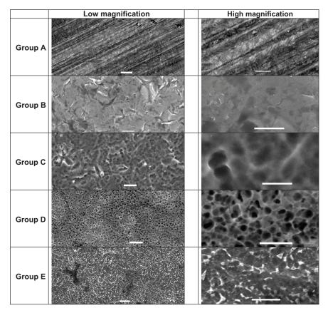
**Figure 2** Scanning electron microscopy images of each sample. **Note:** Scale bars on the left represent  $10 \, \mu m$  and scale bars on the right represent  $5 \, \mu m$ .
