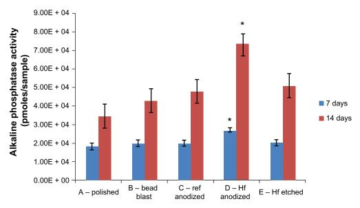
Figure 4 Alkaline phosphatase activity by osteoblasts cultured on the substrates of interest. Notes: Values are represented as the mean  $\pm$  SEM, N = 3. \*P < 0.01 compared to all others at the same time period. For all samples, a significantly (P < 0.01) greater amount of alkaline phosphatase activity was found at increasing time periods.
