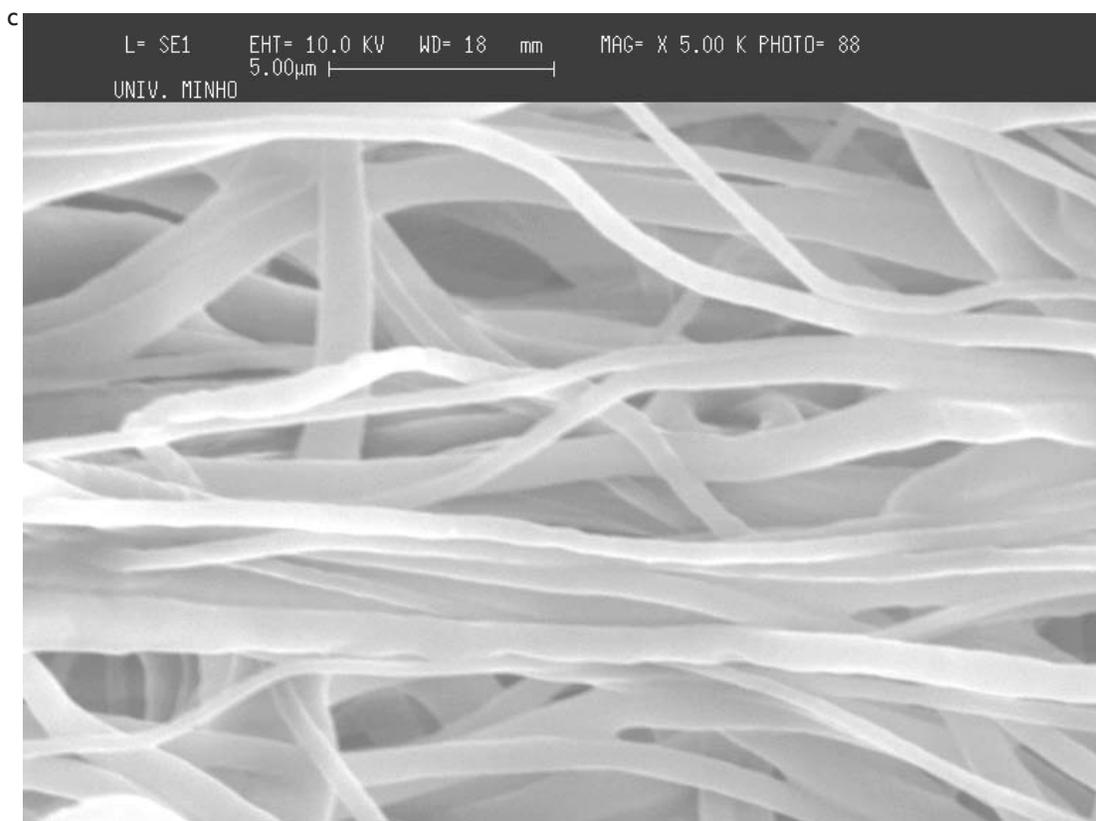
**Figure 7** Deposition of PCL fiber meshes in a metallic wire net: **a)** macroscopic pattern of the fiber mesh, **b)** region of agglomeration of aligned fibers surrounded by random fibers and **c)** aligned fibers
