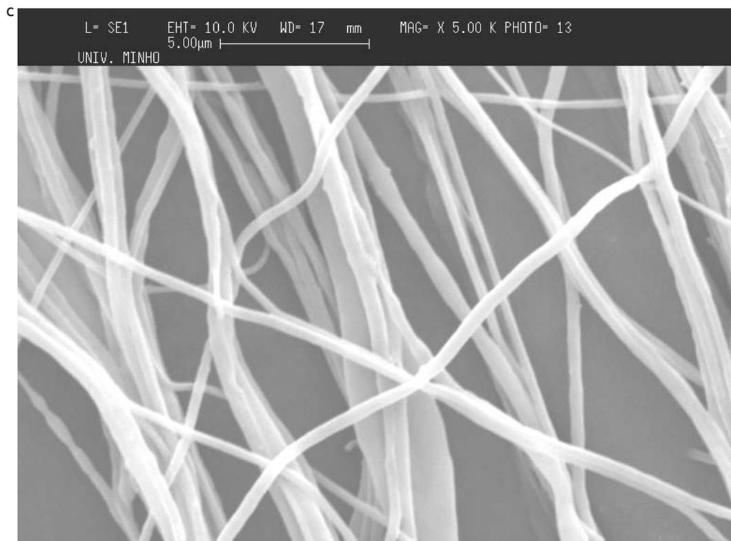
**Figure 5** SEM images of PCL fiber meshes deposited in the screw collector: **a)** lower magnification of the fiber mesh, **b)** close-up showing the region of the mesh corresponding to the thread crest and **c)** the region between two consecutive threads of the screw collector.
