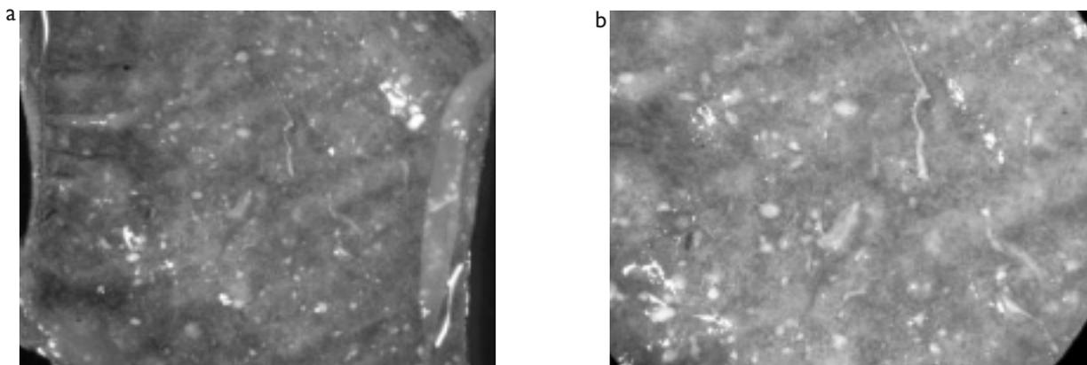
**Figure 10** Stereo light microscope pictures of the cell density and distribution on the surface of PCL fiber meshes obtained with the screw collector stained with methylene blue. a) 25x magnification; b) 50x magnification.
