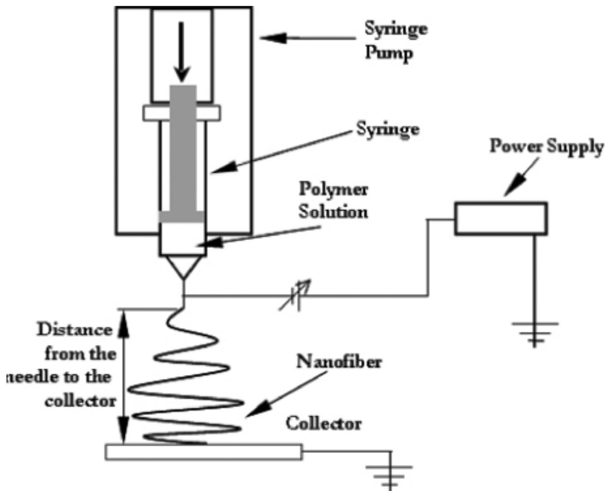
**Figure 2** Schematic draft of the electrospinning apparatus.
