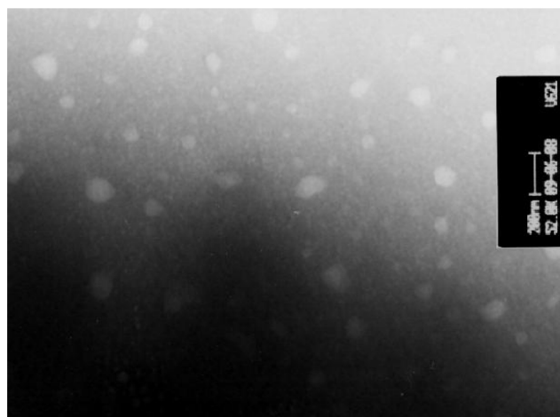
Figure 5 Transmission electron microscopy of probucol microemulsion at the dilution of 1:50 in deionized water.
