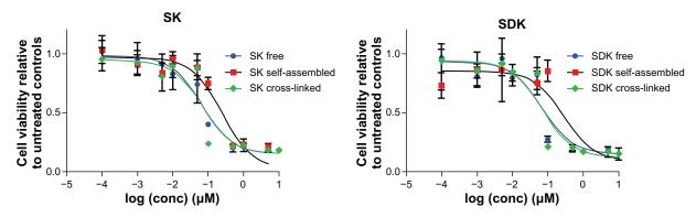
Figure 5 The cytotoxicity of free drug and nanoparticulate formulations for SK and SDK against A549 cell lines. Notes: All points are the average of four measurements  $\pm$  one standard deviation; error bars not visible are obstructed by the point. Abbreviations: SDK, mithramycin SDK; SK, mithramycin SK.
