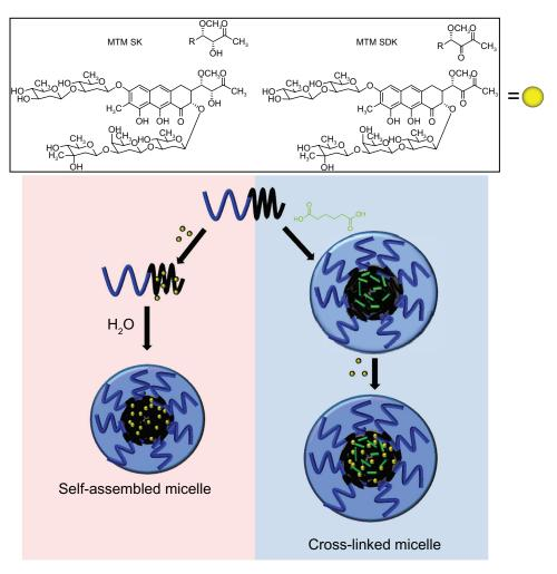
Figure 1 Self-assembled and cross-linked polymer micelles as nanoparticulate formulations for MTM analogs. Abbreviation: MTM, mithramycin.
