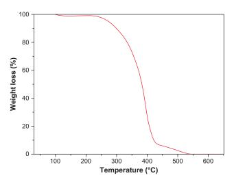
Figure 4 Thermogravimetric profiles of PCL-Tween 80 copolymer. Abbreviation: PCL, poly- $\epsilon$ -caprolactone.
