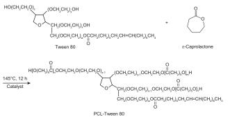
Figure I Schematic diagram of the synthesis of PCL-Tween 80 copolymer. Abbreviation: PCL, poly-ɛ-caprolactone.
