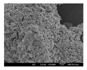
Figure 5 Field emission scanning electron microscopy image of docetaxel-loaded PCL-Tween 80 nanoparticles. Abbreviation: PCL, poly-ε-caprolactone.
