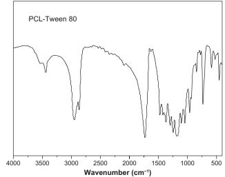
Figure 3 Fourier transform infrared spectra of PCL-Tween 80 copolymer. Abbreviation: PCL, poly-ε-caprolactone.
