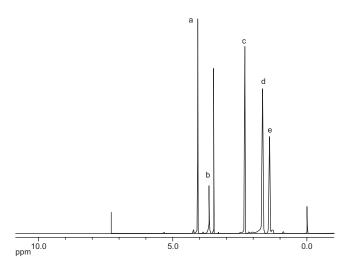
Figure 2 Typical <sup>1</sup>H-NMR spectra of PCL-Tween 80 copolymer. Abbreviations: PCL, poly-ɛ-caprolactone; NMR, nuclear magnetic resonance.
