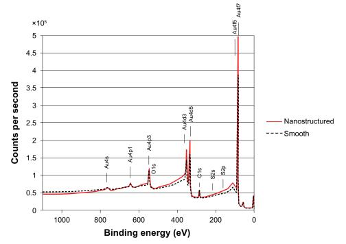
Figure 4 Overlay of X-ray photoemission spectroscopy survey spectra from nanostructured (solid line) and smooth (dotted line) surfaces, showing essentially similar chemical fingerprints.
