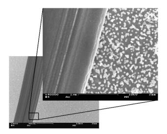
**Figure 2** Scanning electron microscopy images showing a smooth area on a nanostructured gold surface, created by scratching away the particles with a syringe needle. The dark line represents the smooth area. The difference in surface roughness is clearly seen in the magnified inset.
