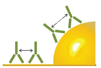
**Figure 9** Illustration of how the curvature of a 60 nm particle affects the distance between adsorbed proteins. In this example, the distance between the CIq binding hinge region of immunoglobulin G molecules are clearly increased by the curvature. (Image drawn according to scale.)
