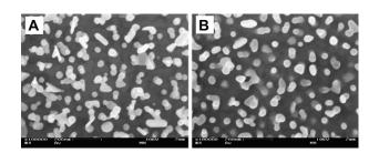
**Figure 3** Scanning electron microscopy images of gold nanoparticles bound to the smooth gold background. (**A**) Particles bound to the surface by electrostatic interaction with a self-assembled monolayer of cysteamine. (**B**) After washing in basic piranha the particles are integrated with the background surface. Magnification: 100,000×.
