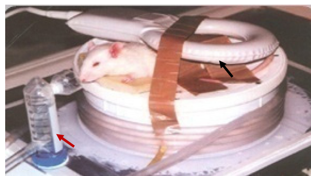
Figure S3 Typical photograph of mouse under magnetic resonance imaging. Red arrow refers to the anesthesia system, black arrow refers to radiofrequency coil.
