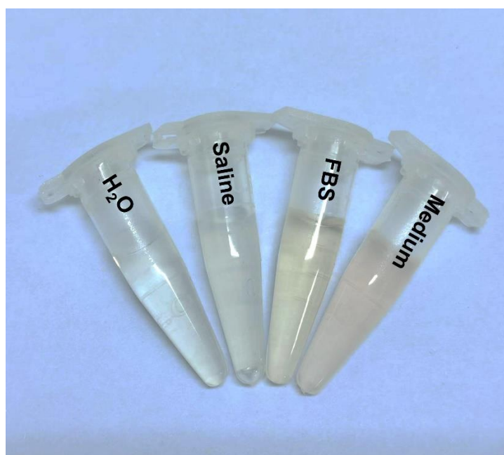
Figure S4. Photograph of FRNPs dispersed in water, saline, serum and cell culture medium.
