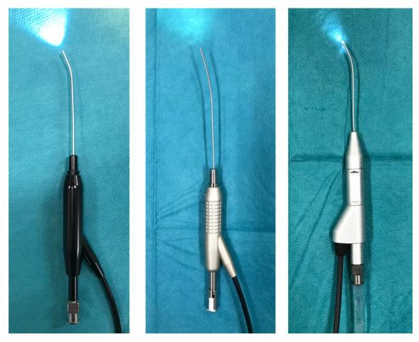
**Left**: CK10 (FiberTech Co., Ltd., Tokyo, Japan); external diameter, 0.9mm; field of view, 60°; image quality, 10,000 pixels
