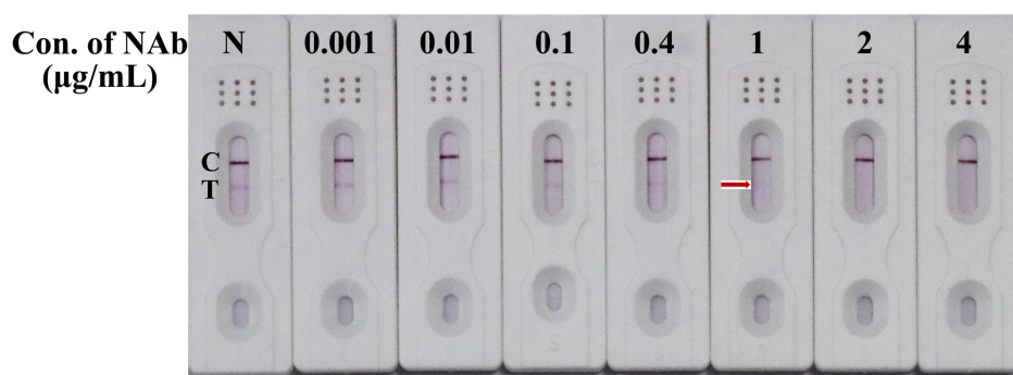
Figure 9 Full image of stability detection of lateral flow kit. Con.: concentration; NAb: neutralizing antibody; N: negative; C: control line; T: test line; Red arrow: Indicates a colour result.
