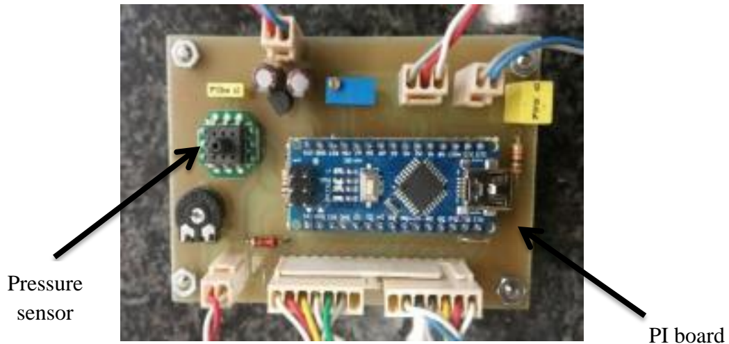
Figure SI5: PCB Circuit of the Proportional-Integral (PI) controller
